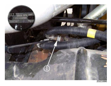
The steering gear information tab is located on top of the steering gear. The sixdigit date code is located on the bottom of the steering gear tab. Refer to the illustration above. The view is from the left (driver's side) of the engine compartment.
