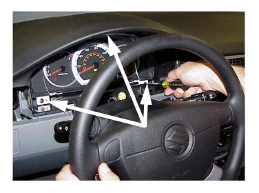
Slide instrument cluster forward enough to remove the three electrical connectors. Then remove and set the instrument cluster aside.
