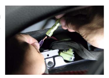
11. Fully crimp the connector using the ratchet crimper. Note the crimper will release automatically if crimped properly.
