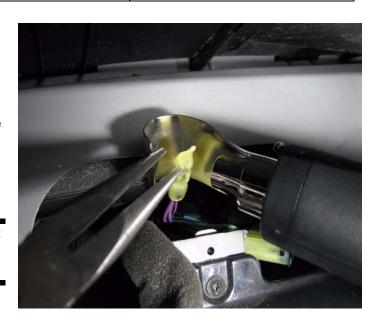
14. When the solder has melted you will see the centering ribs on one side of the crimp connector and the glue should start coming out around the wires.
