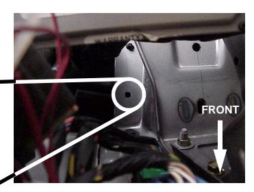
7. Back up at the instrument panel opening, pull the splice pack out from in between the A/C duct and dash support structure. Inspect the splice pack for the three violet wires shown. If present continue to step 8. If they have been cut off, a repair attempt has been made which will have to be removed and then repaired as described starting with step 8.
