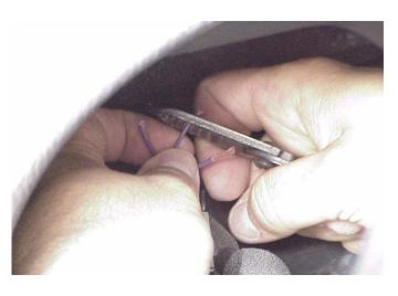
10. Insert the twisted wire end fully into the specified crimp connector. The exposed copper wire should be completely inserted in the metal barrel of the crimp connector. The wire insulation should be inside of the clear area of the connector touching the barrel.
