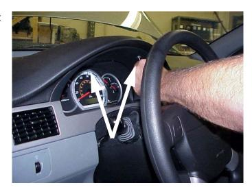
The bezel is secured along the bottom with clips. Some force is required to release clips. Remove the bezel by sliding towards you and tilting up behind steering wheel.
