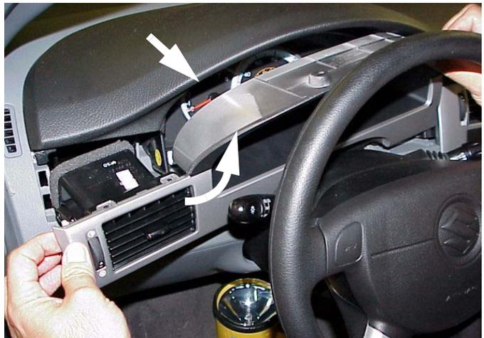
3. Remove the three instrument cluster screws.
