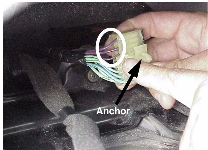
8. Cut the three violet wires just behind any heat damage if it exists. If a repair has already been attempted remove the repair by cutting the wires as close to the repair as possible.
