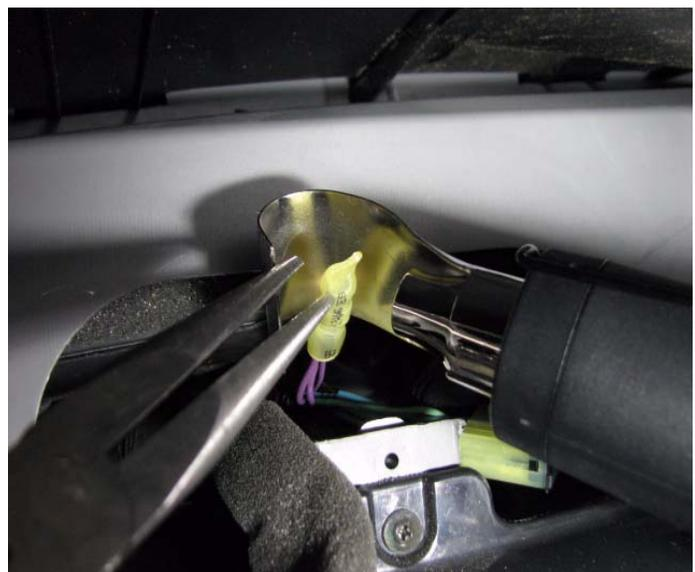
14. When the solder has melted you will see the centering ribs on one side of the crimp connector and the glue should start coming out around the wires.
