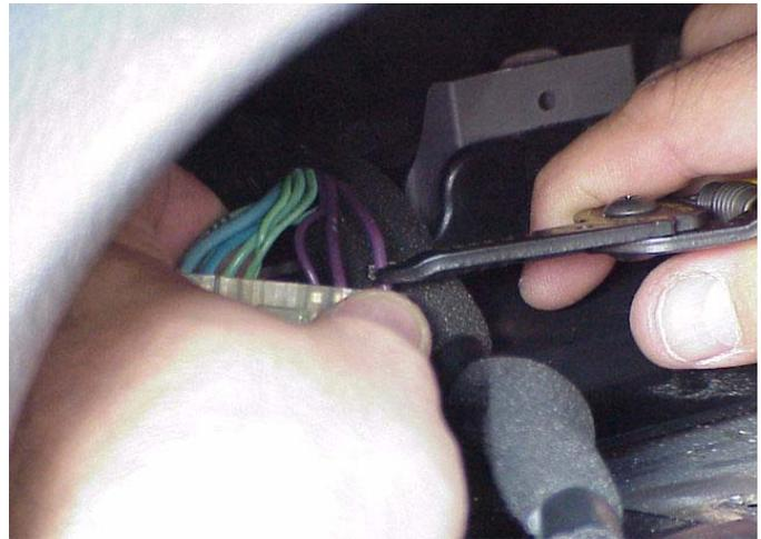
9. Strip about half an inch of insulation off the end of each violet wire and twist the stripped ends together. (It may be necessary to remove some of the harness wrap to expose enough of the violet wires to work with.)
