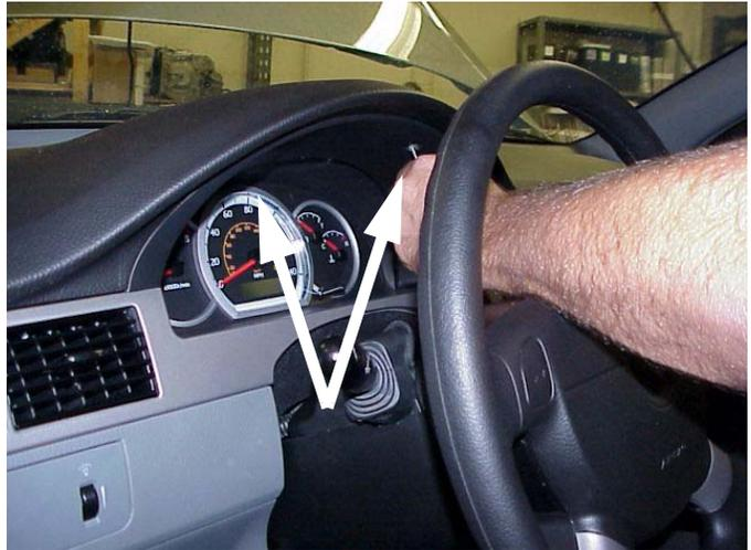
2. The bezel is secured along the bottom with clips. Some force is required to release clips. Remove the bezel by sliding towards you and tilting up behind steering wheel.
