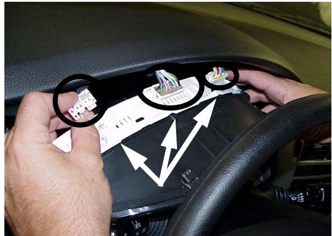
16. Turn ignition OFF. Disconnect battery negative cable. Remove instrument cluster.
