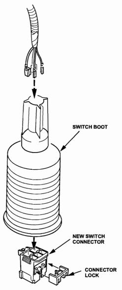
Remove the connector lock from the side of the new switch connector, then insert the terminals into their correct locations in the connector. Reinstall the connector lock.  Pull the switch wires until the connector is in the small end of the switch boot. Using about 10 inches of electrical tape, tape the wires to the boot as shown.
