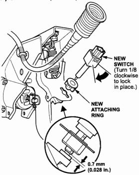
Slide the switch boot over the switch, and connect the switch connector.
