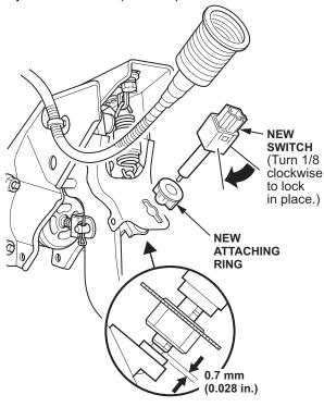
12. Slide the switch boot over the switch, and connect the switch connector.
