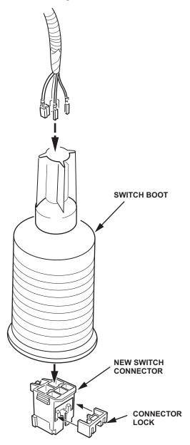
9. Remove the connector lock from the side of the new switch connector, then insert the terminals into their correct locations in the connector.
