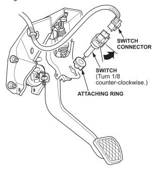
4. Note the terminal locations and wire colors in the switch connector. You'll need to install the terminals in the same locations in the new connector. Depending on the model, the connector has two or four terminals. The terminal locations are listed below.
