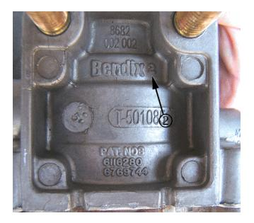
b. If the casting has "Bendix 2" (2) on the stud side of the air brake park control valve, proceed to the *External Check Valve Service Kit Procedure* below.
