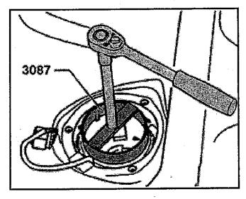
Secure closing flange with locking ring using 3087 wrench or T10202 and tighten to 145 Nm (106 ft. lbs.)
