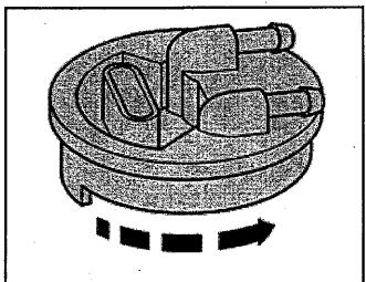
When installing closing flange, turn in direction of arrow, as shown in illustration
