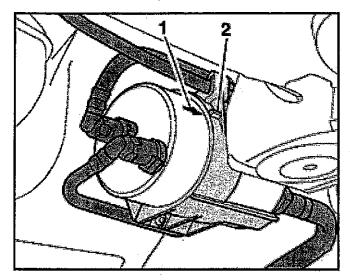
Install new fuel filter (8E0 201 511 J) into bracket
