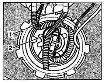
Ensure that wiring for fuel pump -2- and fuel return line -1- is correctly routed when installing closing flange
