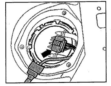
Carefully release 4-pin harness connector -arrow- and disconnect
