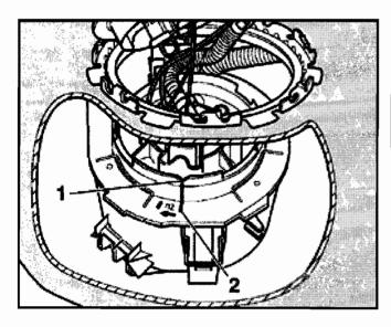
Remove fuel delivery unit from baffle housing when notch -1- is aligned with mark -2-
