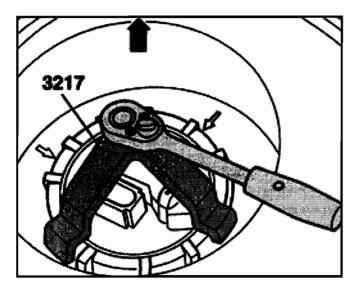
Secure closing flange to fuel tank with union nut and using ring nut spanner tool 3217, tighten to 80 Nm (59 ft. lbs.)
