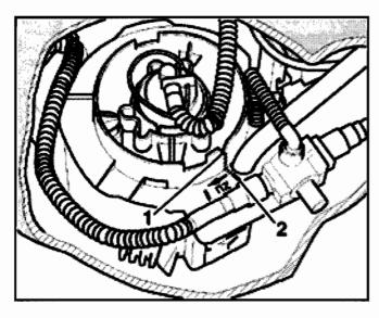
Remove fuel delivery unit from baffle housing when notch -1- is aligned with mark -2-
