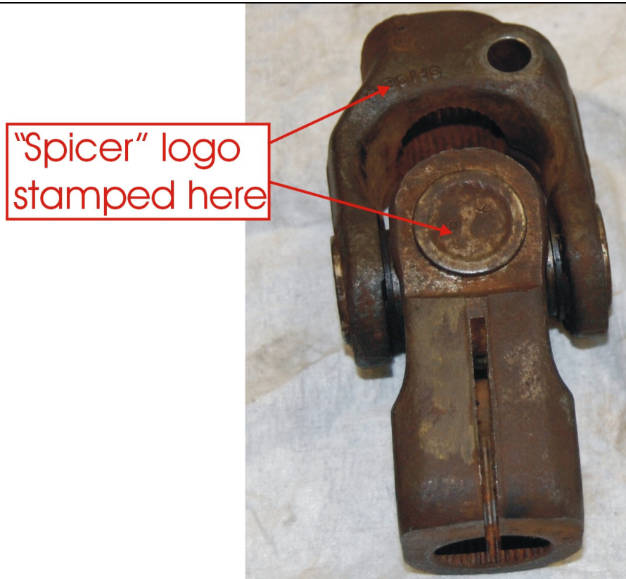
Figure 2: U-Joint assembly requiring replacement.
