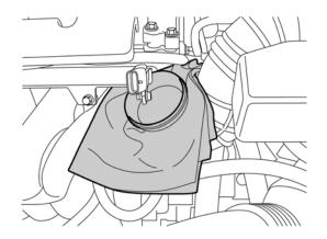
Position paper under the fuel pressure sensor to catch any gasoline remaining in the fuel rail.
