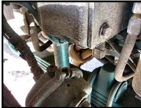
Figure 1; Hood support & brake chamber "before" repairs
