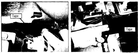
**8.** Reinstall the floor carpet. Wrap the previously cut portion of carpet with 1.5 inch wide unwoven adhesive tape.
