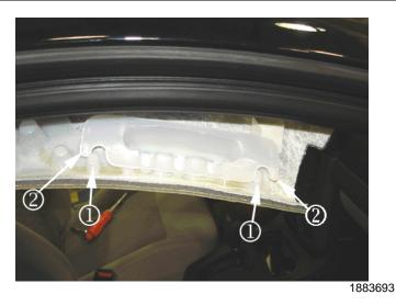
**Important:** Ensure that the energy absorbing (EA) plastic piece is installed properly. The tail ends of the energy absorbing (EA) plastic piece (2) should wrap around the anchor posts (1) of the headliner material. The body of the EA plastic piece should be firmly attached to the headliner.
