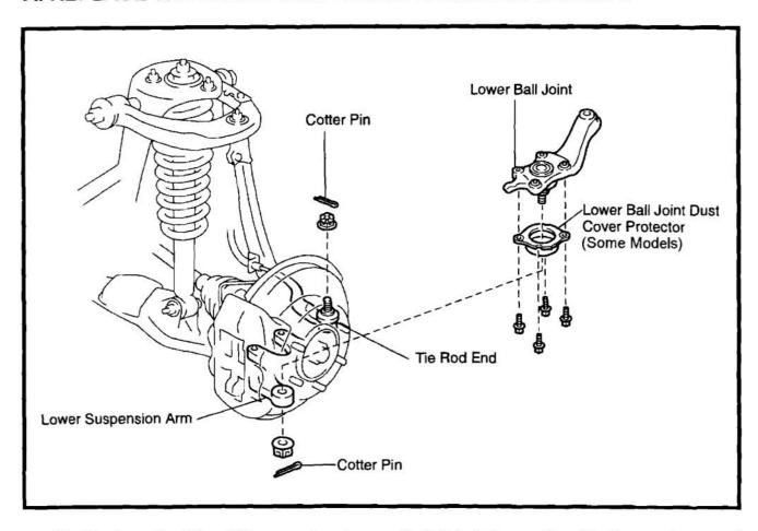
Replace the "Front Suspension Lower Ball Joints" as outlined in the repair manual (TIS keyword: "Front Lower Ball Joint Removal & Front Lower Ball Joint Installation".)
