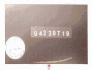
Please refer to the 8-digit lot # code immediately following the part number '20-6644-00' near the bottom of the label to determine manufacture date. The 8-digit code = Month, Day, Year, Hour (MMDDYYHH). The example above was manufactured on April 23<sup>rd</sup>, 2007 at 19:00 hour.
