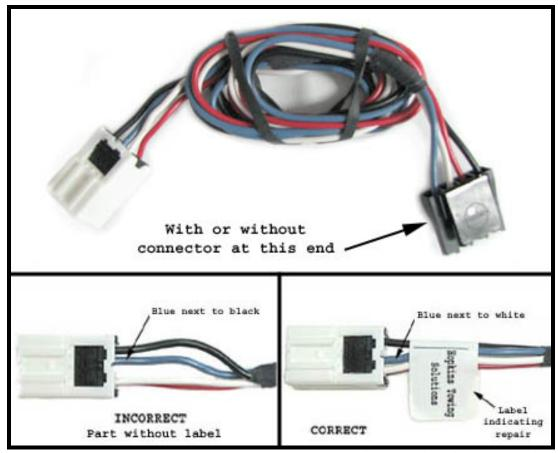
Harnesses sold between July 2006 and June 2007 may have a wire placed in an incorrect location. This could result in improper trailer braking when the towing vehicle brakes are applied, possibly leading to personal injury, and/or property damage.
