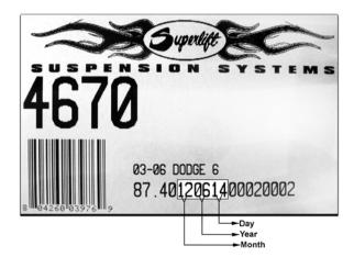
**SAMPLE KIT BOX LABEL:** Referencing the packaged date may help identifying suspect parts. Affected pitman arms were packaged between approximately 9/21/05 and 1/16/07. Superlift<sub>®</sub> packaged date begins with the 5<sup>th</sup> digit of the label. For example, this pitman arm was shipped 12/14/06. Additionally, pitman arms are identified by a paint stripe. Affected arms have a purple stripe; new edition arms have a gold stripe.
