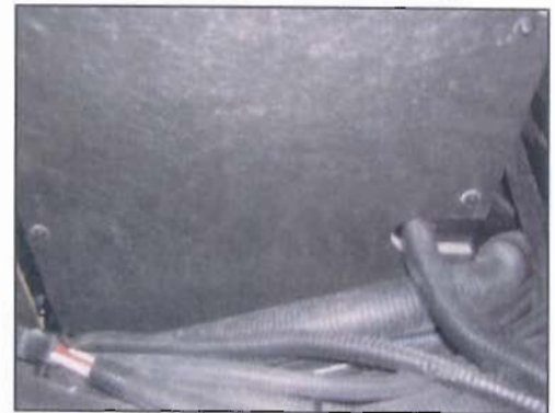
FIGURE 12 Cut openings for wire harnesses in Water Fill Compartment Bottom as necessary.
