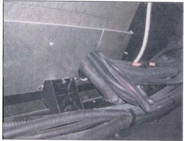
FIGURE 6 Install the two pieces of Polyurethane material so that the wire harness passes through the hole cut in Step 24.
