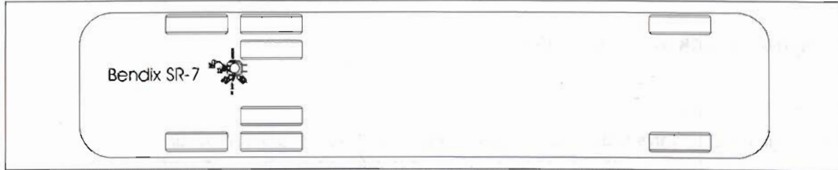
FIGURE 1: BENDIX SR-7 LOCATION ON H3, X3 AND XLII MTH SERIES VEHICLES (TYPICAL)
