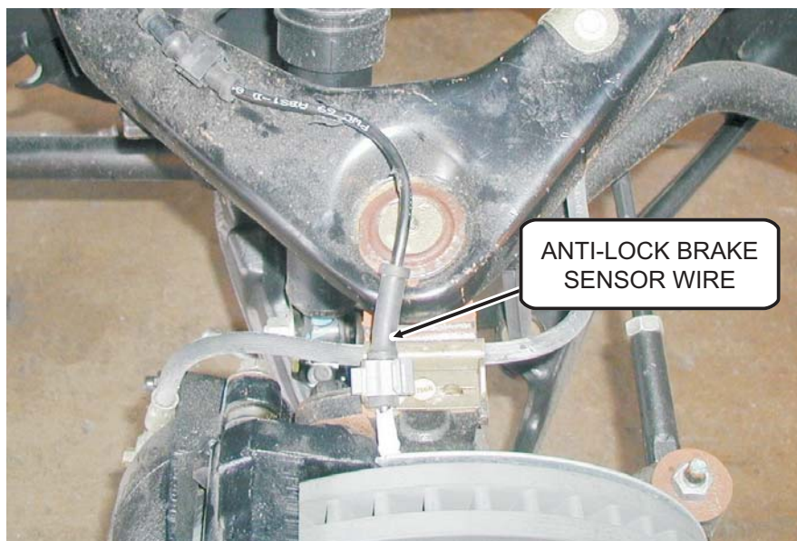
FIGURE 6 ANTI-LOCK BRAKE SENSOR WIRE IN NEW LOCATION
