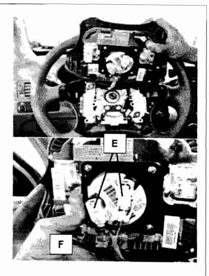
5. Remove the four air bag inflator fixing bolts from the existing air bag module.
