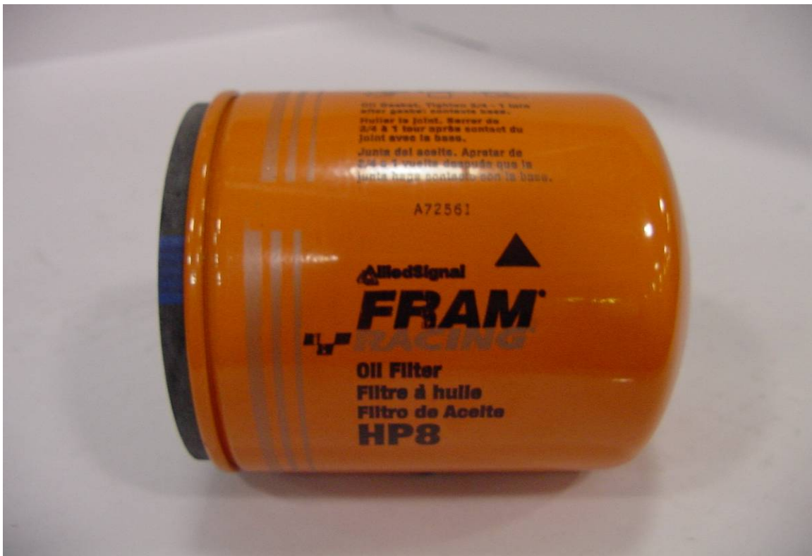
The part number (HP8) and the date code (eg. A72561) are found on the side of the oil filter.
