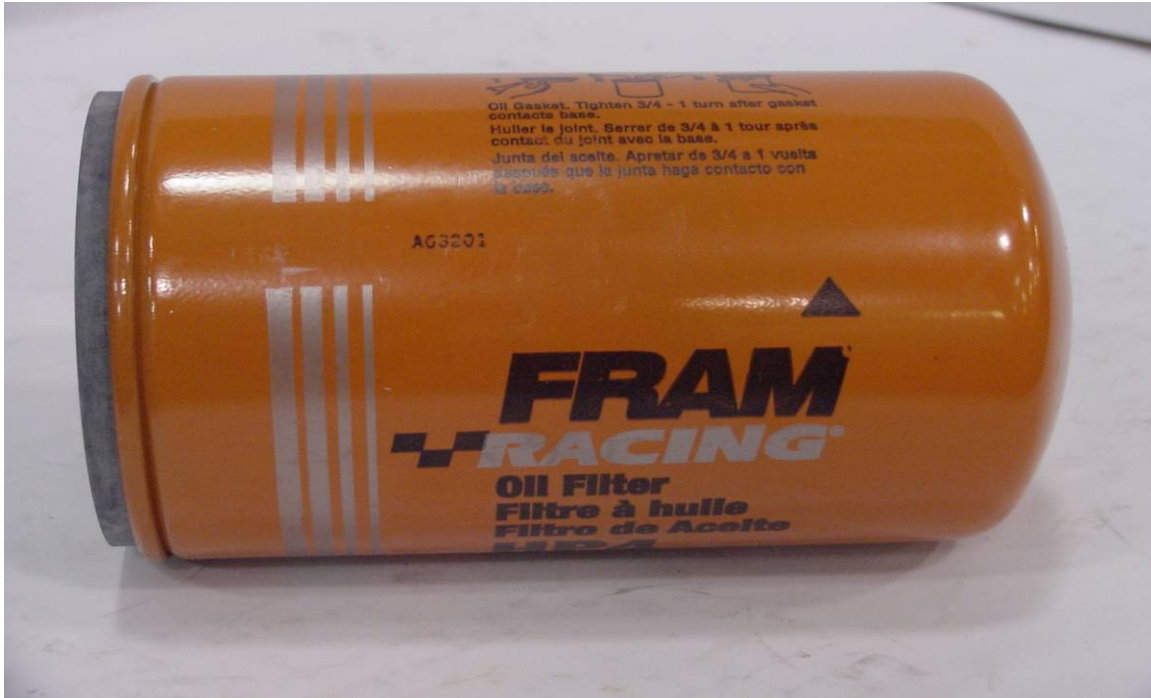
The part number (HP4) and the date code (eg. A63201) are found on the side of the oil filter.
