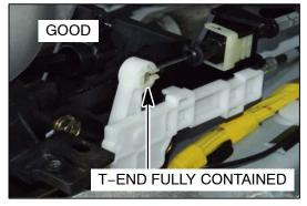
If the cable end is fully contained within the lever and snap lock, the cable DOES NOT need to be replaced.
