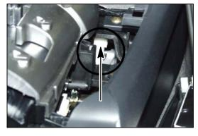
7. Inspect the T-end of the gear shift key interlock cable as described below.
