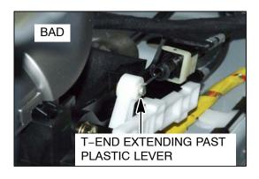
b. If the T-end of the cable is visible (flush or extends past the white plastic lever), the cable must be replaced.
