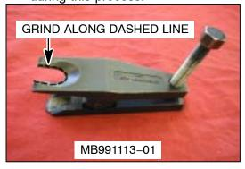
**NOTE:** If special tool MB991113-01 – ball joint remover is used, it will need to be modified. Grind the opening, in the area shown, just large enough to go around the ball joint.
