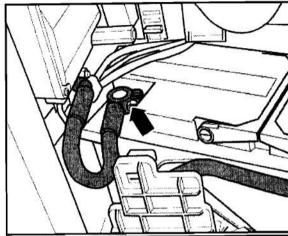
□ Disconnect battery ground (GND) cable -arrow-
