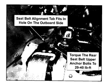
\*NOTICE Install the Lower Seat Belt Anchor With the Buckle Tongue Facing Forward, Without Twists in the Webbing.
