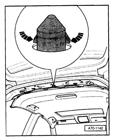
Disengage retainer at rear retaining clip -arrows- using small hook tool
