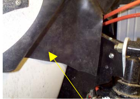
Remove plastic rivet
