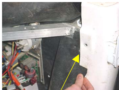
Tuck shield under body side panel
