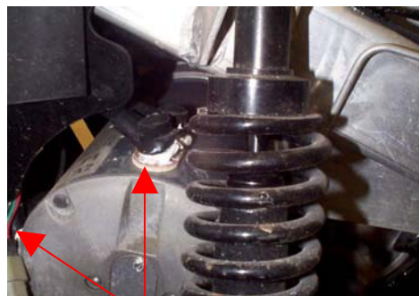
Field & Armature studs
