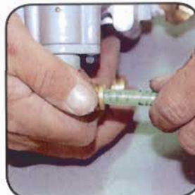
To connect the airlines, push the line inward until it bottoms.
