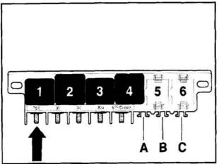
Connect jumper wiring harness wire -#9-(yellow/black) to micro central electric contact 75X -arrow-, tighten to 9 Nm (79 in. lbs.)
