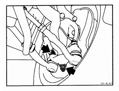
tightened to a torque of 165 Nm.
