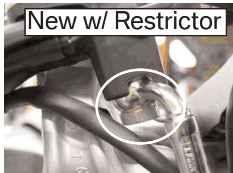
Fig. 1: New banjo bolt with restrictor is a hex head design. (K - Model shown)
