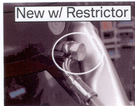
Fig. 1: New banjo bolt with restrictor is a hex head design. (R - Model shown)
