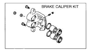
c. Using the new caliper and bolts provided in the brake caliper kit listed in the PARTS INFORMATION section of this bulletin:
