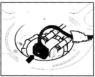
Carefully release 4-pin harness connector -arrow- and disconnect
