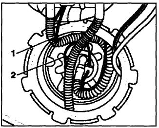
Ensure that wiring for fuel pump -2- and fuel return line -1- is correctly routed when installing closing flange
