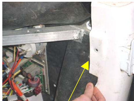
Tuck shield under body side panel
