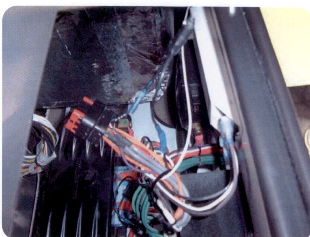
CHECK IF WIRE IS CRIMP OK AND APPLY HEAT TO CONNECTOR.
