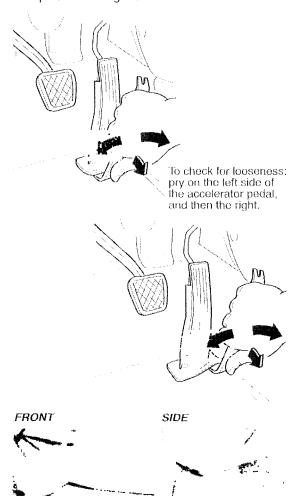
Pedal edge will bend if the pedal is secured.
