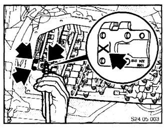
8. Install the new guide plate (PN 24 53 1 219 287) and tighten four guide plate bolts to 10 Nm.
