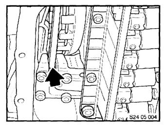
wheel and the pawl is not sticking/binding in the guide plate (check point indicated by an arrow. 11. Install a new transmission oil pan seal/gasket. On E60/63/64/65/66 vehicles, also replace the transmission pan sealing O-ring (PN 24 11 7 520 714).
