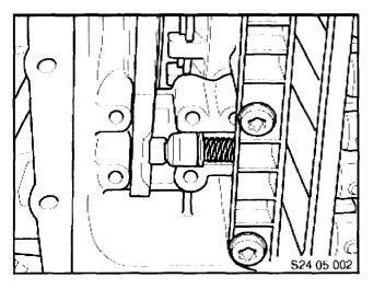
7. Remove the parking pawl guide plate (illustration shows guide plate removed from the transmission).
