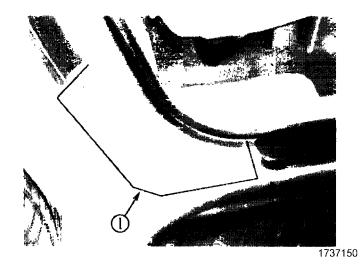
1. Ensure that the rear rocker panel in the tape contact area (1) is clean and dry. Use a non-oil based cleaner, preferably isopropyl alcohol. For Chevrolet TrailBlazer EXT with molded-in-color rear rocker, coat the top of the rocker with adhesion promoter, P/N 12378462-U.S., 10953554-Canada, or equivalent, and then allow it to dry.
