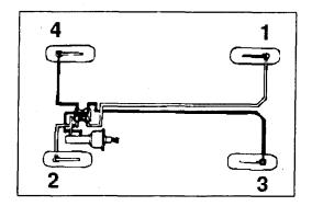
21. Start the engine and bleed the air in the brake lines at each caliper, in the sequence shown.
