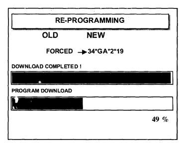
6. When the "REPROGRAMMING COMPLETED" message is displayed, turn the ignition key to the OFF position. Wait at least 3 seconds and then re-install the current system software card to the Hi-Scan Pro. Inspect the indicator lights as described on scan tool screen. All indicator lights should be OFF.
