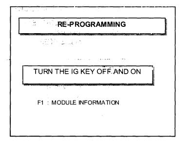
5. The Hi-Scan Pro will reprogram the ECU manually. (See the ROM ID table on the front page for previous and new ESP module ROM ID's.)
