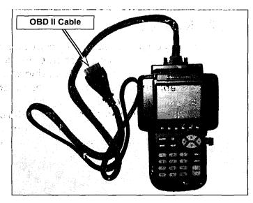
Connect the OBD-II Data Link Connector (DLC) cable under the dashboard on the driver's side.
