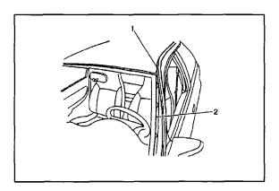
66. Reposition the front door sealing weatherstrips (1) to the pinch-weld flange.
