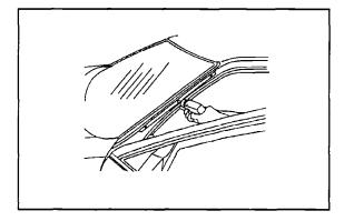
65. Install the windshield side reveal moldings screws. **Tighten**
