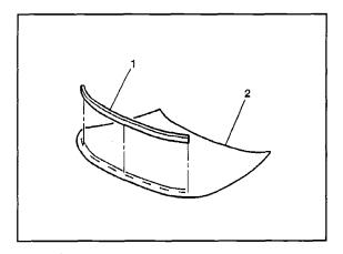
41. Install the new windshield acoustic strip (1) to the windshield (2), if equipped or damaged. The acoustic strip aids in reducing noise.
