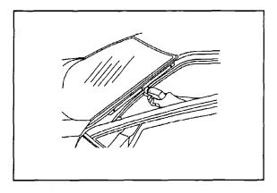
15. Remove the side reveal molding screws.
