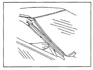
16. Remove the side of the reveal moldings.
