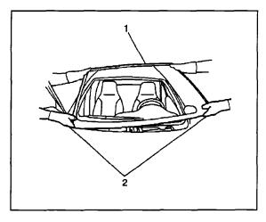
43. With the aid of an assistant, dry fit the window (1) to the opening in order to determine the correct position.
