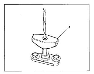
3. Use the tool (1) provided with the vehicle to unscrew the antenna mast, if equipped.
