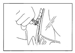
IMPORTANT: Keep the cutting edge of the tool against the window.
