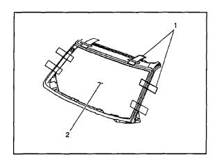
55. Align the masking tape (1) lines on the window (2) and the body.
