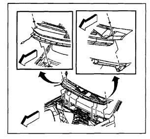
68. Position the air inlet grille panel to the rear edge of the hood.
