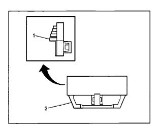
IMPORTANT: The windshield lower supports (1) have molded in locks with an adhesive strip (2) on the backside. If the windshield lower stops have been removed, they must be replaced.
