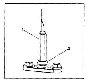
IMPORTANT: Install the antenna mast using the mast tool. Ensure the antenna mast is fully seated to the antenna base.
