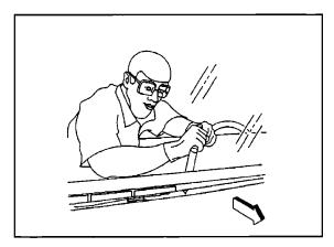
30. Remove the bottom of the windshield from the urethane adhesive using a long utility knife or similar tool. Keep the cutting edge of the utility knife against the glass. Do this from inside the vehicle.
