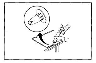
51. Cut the applicator nozzle in order to provide a bead of 12.7 mm (1/2 in) wide and 12.7 mm (1/2 in) high.
