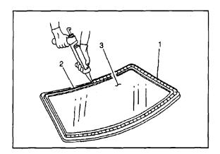
53. Use the edge of the window or the inside edge of the reveal molding as a guide for the nozzle in order to apply the urethane adhesive (1) to the inner surface of the window (3).
