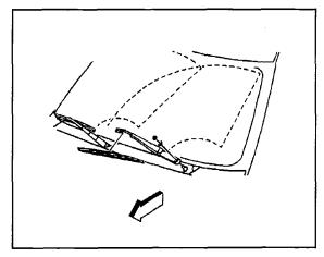
73. Install the wiper arm onto the drive shaft.
