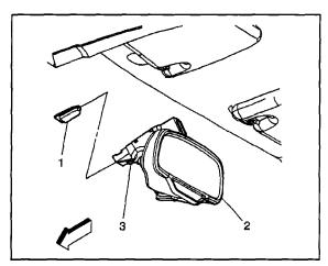
79. Slide the mirror (2) onto the support button (1).
