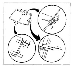
42. If installing a new window reveal molding, start in the center and work toward each end pressing firmly into place.
