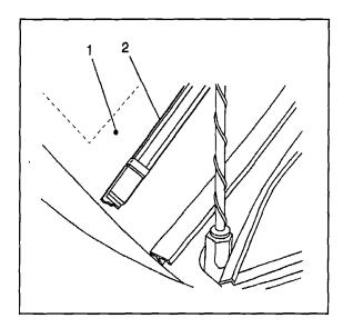
74. Hold the wiper arm blade (2) in position to the dots (1) in the windshield blackout area.
