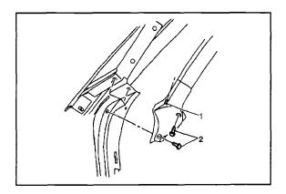
67. Install the push-pin retainers (2) to the front door sealing weatherstrips located at the base of the windshield pillar.
