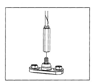
77. Install the antenna mast to the antenna base, if equipped.
