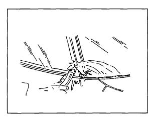
IMPORTANT: Do not direct a hard stream of high pressure water to the freshly applied urethane adhesive.
