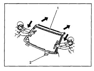
54. With the aid of an assistant, place the window in the opening. Place the windshield on the lower supports (2), if equipped.
