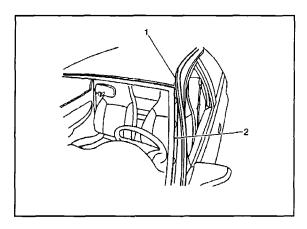
14. Reposition the front door sealing weatherstrips (1) in order to access the side reveal molding screws. It is not necessary to remove the front door sealing weatherstrip completely from the vehicle.
