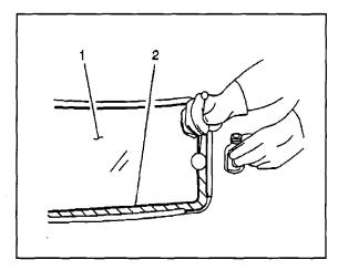
IMPORTANT: The glass primer black #2 is effective up to 8 hours after applying it to the glass. The primed surface of the glass must be kept clean.
