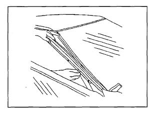
64. Install the windshield side reveal moldings.
