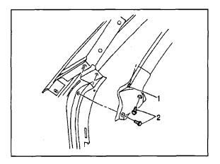
13. Remove the push-pins (2) from the front door sealing weatherstrips (1) located at the base of the pillar.
