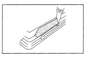
52. Use a cartridge-type caulking gun in order to apply a smooth, continuous bead of urethane adhesive.
