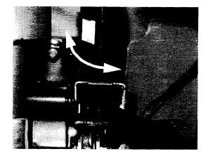
10. With the plunger still at its maximum extension release the pedal slowly until it contacts the head of the plunger of the brake light switch.
