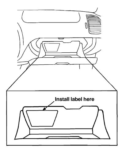
2. Wipe the area where the warning label will be affixed with a clean, dry cloth to remove any dust or dirt.
