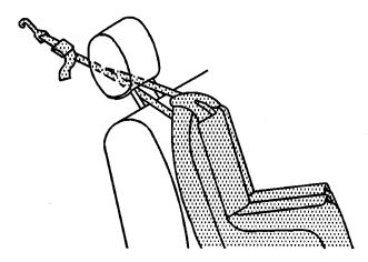
If the position you are using has a head restraint and you are using a dual tether, route the tether under the head restraint and in between the head restraint posts.
