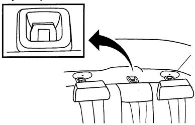
Your vehicle has top strap anchors for the rear seating positions. The anchors are located on the filler panel behind the rear seat head restraints.
