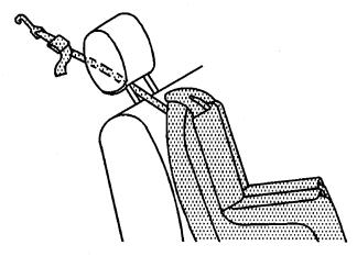
If the position you are using has a head restraint and you are using a single tether, route the tether under the head restraint and in between the head restraint posts.
