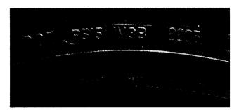
Tires made for use in the United States have the DOT serial number located on one sidewall of the tire near the rim. Starting with the year 2000, four numbers are used for the Date of Manufacture. The first
