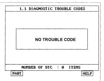
8) When the reprogramming and erasing DTC is completed successfully, turn the ignition key to the off position and then start the engine to check for proper operation.
