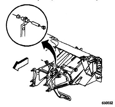
3. Remove the brake pedal nut and bolt.
