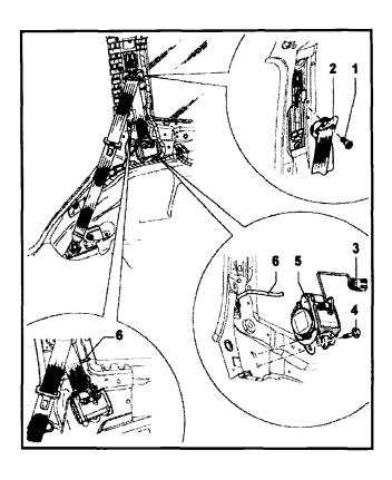
Remove bolt -1- and pull belt relay -2- off belt height adjuster
